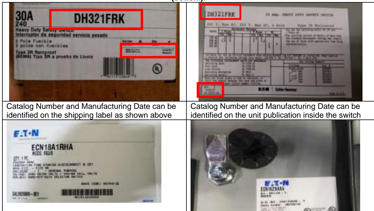
Figure 1. Location of catalog number and date code for safety switches (top) and enclosed control (bottom).
