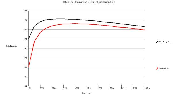
Figure 3. New, energy-efficient transformers provide the greatest advantage under real-world load levels.
